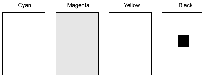
Figure 13.4 Color separations for a simple image, with black overprinting
